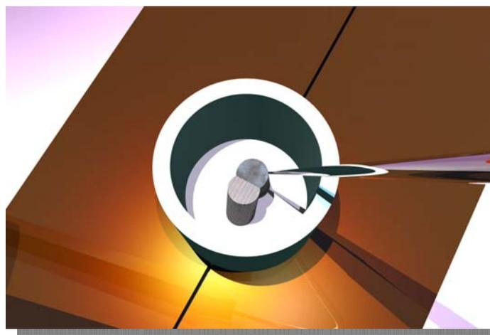
4.1.8 As discussed earlier the first weld process involves discharging energy from a capacitor bank through the weld arc. This can be done on all cable sizes from 1.0mm to 6.0mm however there is a considerable energy discharge when welding 6.0mm cable conductors using capacitance discharge. If necessary welds of 6.0mm cable conductors can be carried out using straight TIG and this procedure will be dealt with later. (Welding 6.0mm using capacitance discharge will not damage the machine)
