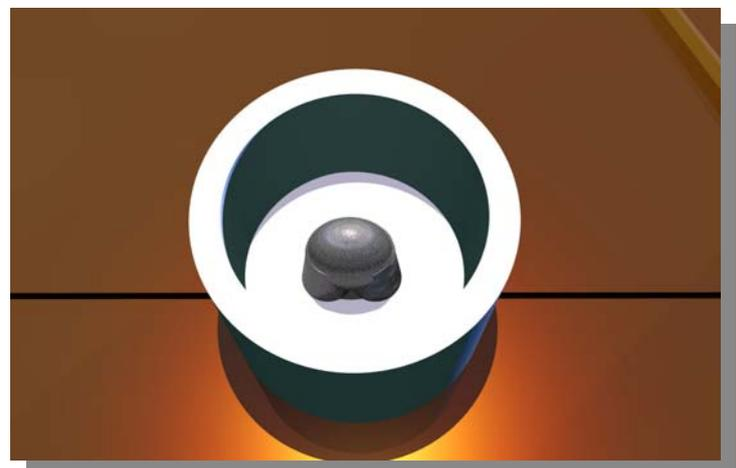
**4.2 The next part of the procedure involves using caps and back-filling powder. Many thermocouple manufacturers do not use either items and the procedure goes directly to the finished weld from here. However some specifications demand the use of caps and back-filling powder especially for the larger cable sizes. The instructions that follow assume that this is the case.**
