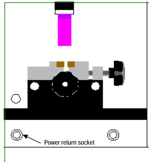
4.3.4 When welding the sheath of 6mm cable, the mass of material involved means that some distortion occurs in the weld pool during the process. The end result requires some degree of cleaning-up such as extensive grinding. The ground tip may appear to be adequate but there is no certainty that there is enough material to form a serviceable weld.
