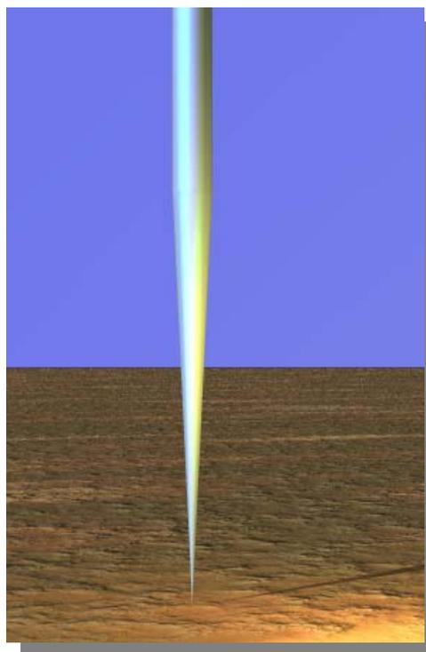
A good trick to determine if the electrode is sharp enough is to run it lightly over your thumbnail. If the point digs in it is sharp if it slides it needs a little more grinding.
