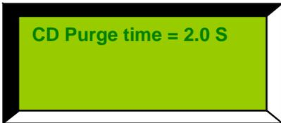
To check the CD Purge time set the weld mode switch to Standby then press the CD START and CD STOP buttons together and hold. The display will be as shown.
