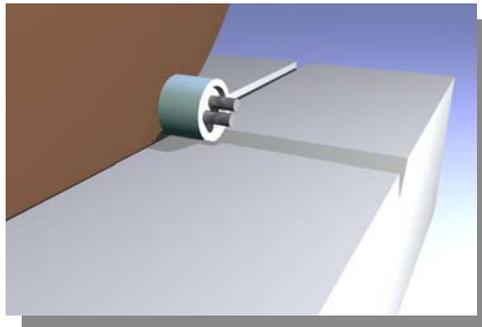
4.1.4 **Drill** the cable end using the Precision MI Drilling jig. (Instructions for operating drilling jig are given in Appendix 2)
