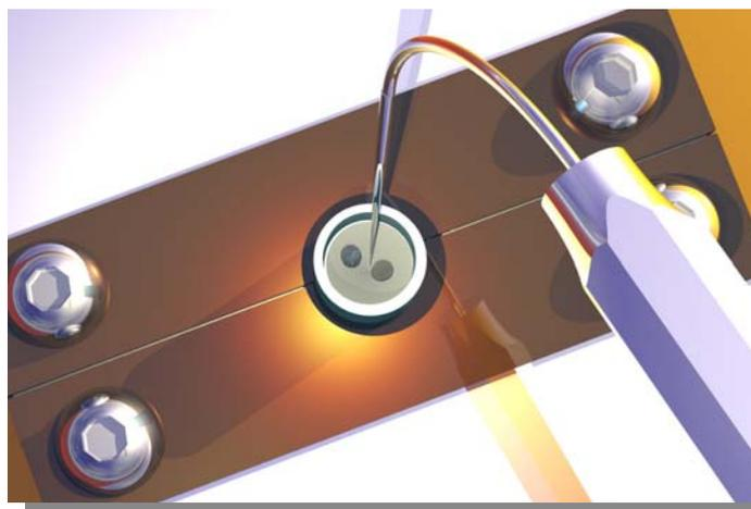
4.1.7 Using the Powder Probe gently push the two conductors together so that they touch along the drilled surfaces. You will need to keep blowing away excess insulation to keep the weld area clean. Once the conductors are in position the first weld process can proceed.
