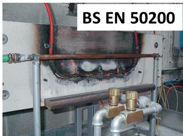
A quick glance at the fixings of these samples during common British Standards tests for fire rated cables shows clearly the massive disparity between how cables are tested and approved and how fire rated cables are actually installed.
